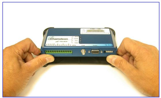
Installing the modem in its base.
